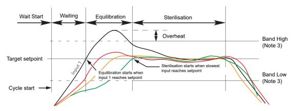
Figure 42 Steriliser cycle
