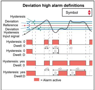
Figure 95 Deviation alarm parameters
