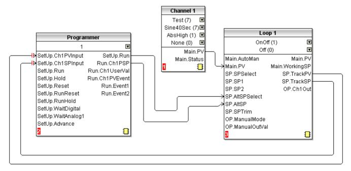
Figure 120 Programmer to Loop basic wiring
