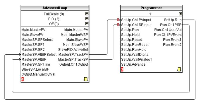
Figure 119 Advanced loop to Programmer basic wiring
