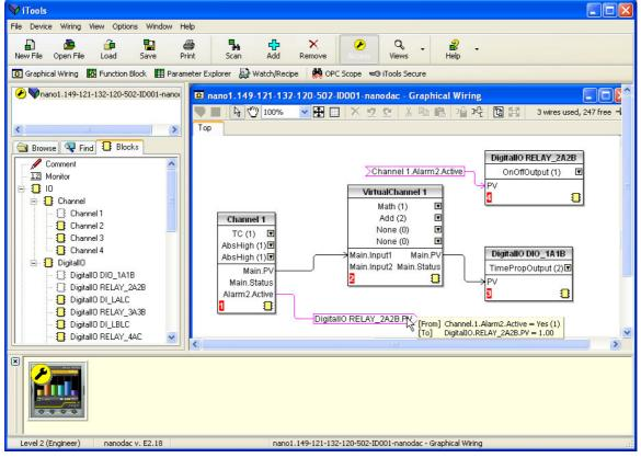
Figure 171 Graphical wiring Editor
