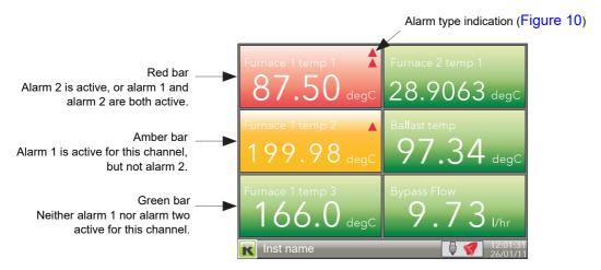
Figure 24 Alarm panel display (six channels)
