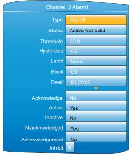
Figure 193 Channel 2, Alarm 1 set up
