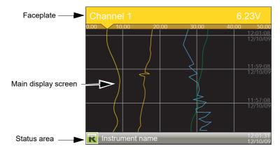
Figure 6 Display mode screen (vertical trend)
