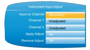
Only those channels with 'Type' set to 'Dual mA', 'Dual mV' or 'Dual T/C' appear in the list of secondary channels. In this example, only channels 1 and 3 are configured as dual input. (See "Channel Main" on page 121 for channel Type configuration.)
