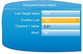
Figure 73 Channel adjustment procedure (2)
