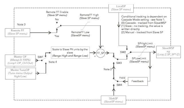
Figure 111 Cascade Full Scale Mode Block Diagram
