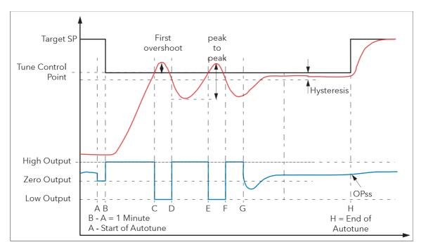
Figure 209 Autotune from below setpoint
