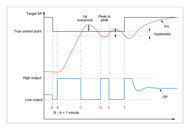
Figure 206 Autotune heat only process (from below SP)
