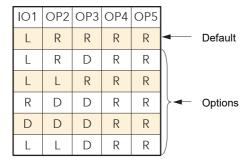
L = Logic output; R = Relay; D = DC output OP4 and OP5 share Common terminals.
