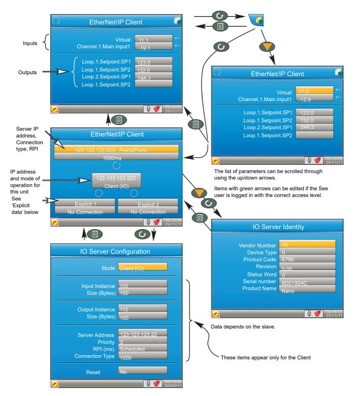
Figure 49 Typical EtherNet/IP display
