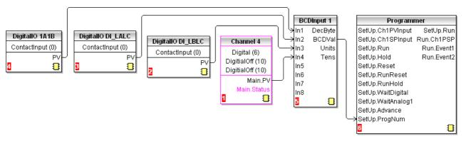
Figure 39 BCD Switch Wiring
