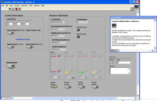
Figure 230 Steriliser Application (showing Context Help)
