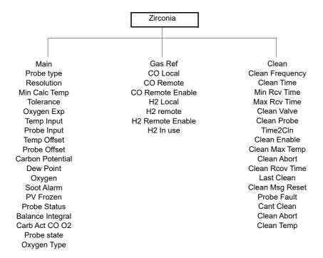
Figure 134 Zirconia probe configuration layout.
