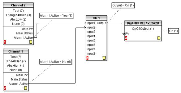
Figure 223 iTools representation of OR block usage
