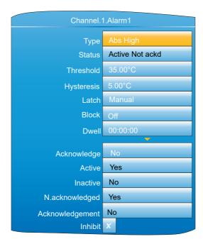
Figure 93 Typical alarm 1 configuration menu
