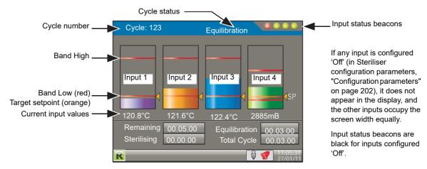
Figure 41 Steriliser display mode (typical) (four inputs)
