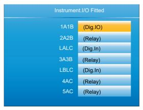
Figure 69 I/O fitted display
