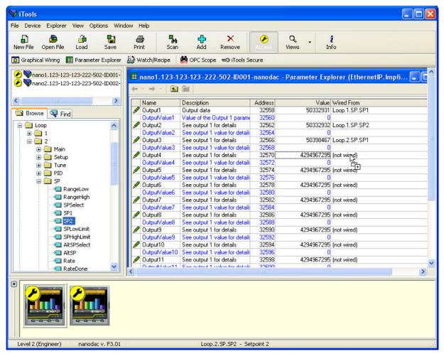
Figure 51 Dragging a parameter to the Output table
