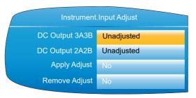
1A1B and 2A2B can be configured only as mA outputs.
