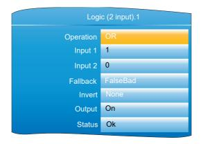
Figure 145 Two-input logic block configuration
