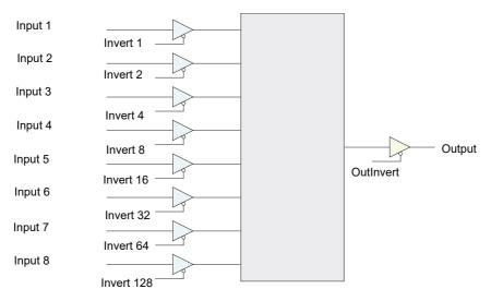
Figure 147 Logic (8 input) block schematic
