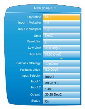
Figure 150 Block configuration (typical)
