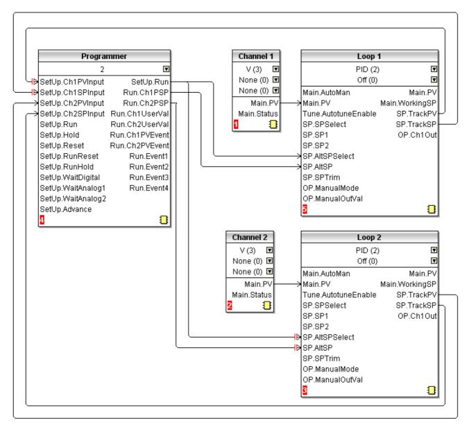
Figure 121 Dual programmer to two loops basic wiring
