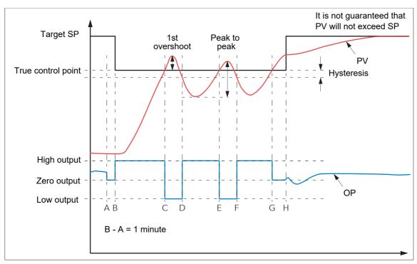
Figure 205 Autotune heat/cool process
