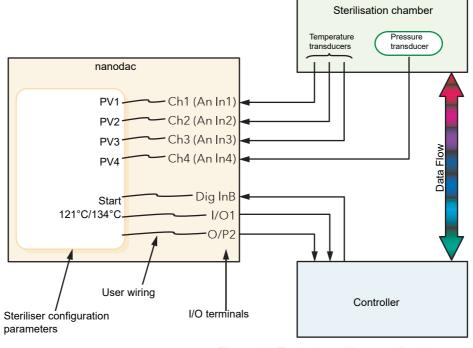
Figure 43 Typical steriliser application
