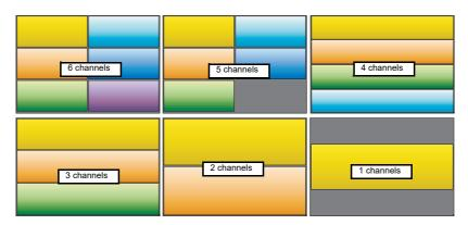
Figure 23 Display layout for different numbers of channels
