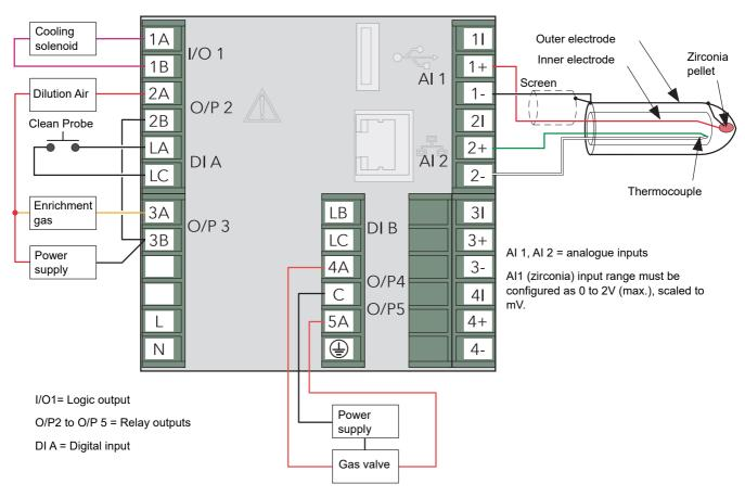
Figure 136 Typical Zirconia probe wiring
