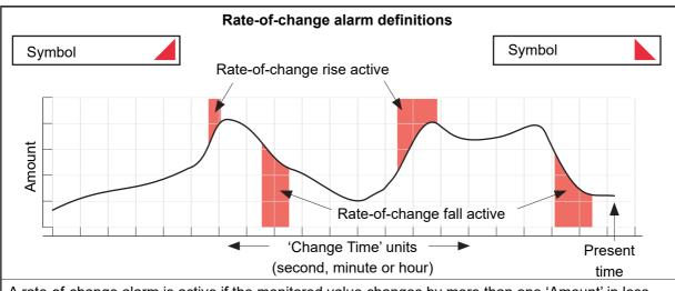
A rate-of-change alarm is active if the monitored value changes by more than one 'Amount' in less than 1 'Change time'. Dwell delays the alarm on-time. Averaging removes the effects of signal noise.
