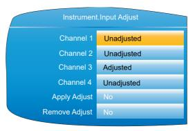
Figure 71 Input adjust top level display
