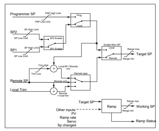
Figure 213 Setpoint Function block
