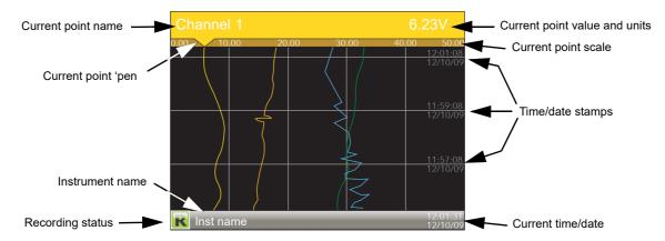
Figure 9 Typical display screen (Vertical trend)
