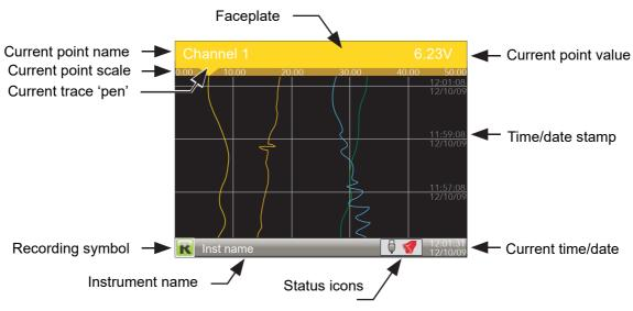
Figure 18 Vertical trend mode display elements
