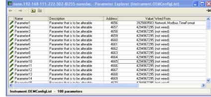
Engineer level when OEM security is enabled. In this example the parameter 'TimeFormat'.
