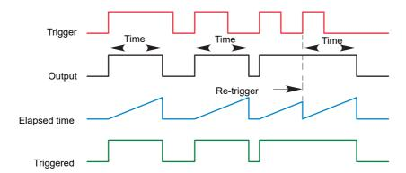
Figure 153 'On Pulse' definitions ON DELAY
