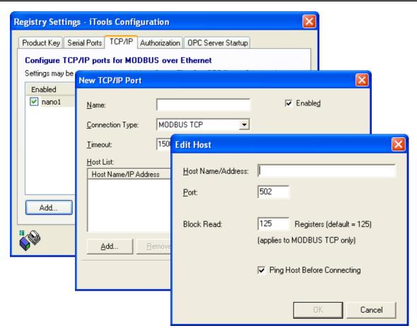
Figure 166 Adding a new Ethernet port
