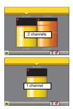
Figure 20 Vertical bargraph display mode
