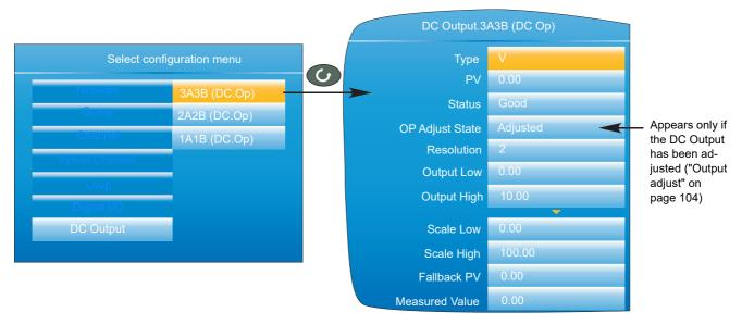
Figure 132 DC Output option configuration page (typical)
