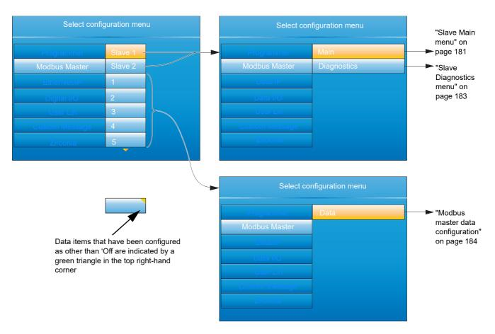
Figure 122 Modbus Master configuration top level menus
