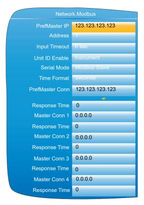
Figure 84 Modbus TCP configuration menu
