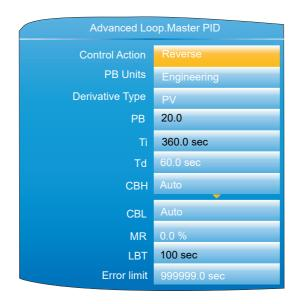
Figure 107 Advanced Loop master PID menu
