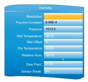
Figure 142 Humidity calculation configuration
