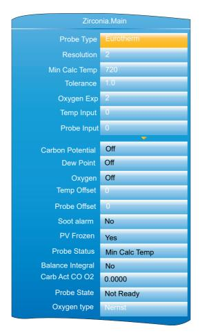
Figure 135 Zirconia Probe configuration (typical)
