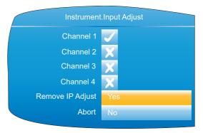
Figure 75 Channel adjustment removal
