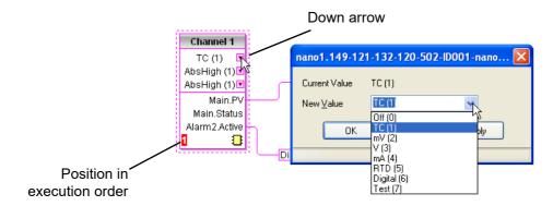
Figure 172 Function block example
