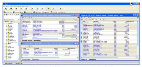
Figure 192 OEMStatus parameter set to 'Locked'
