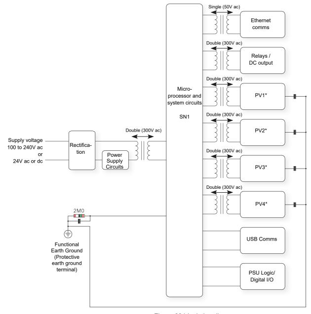
Figure 224 Isolation diagram
