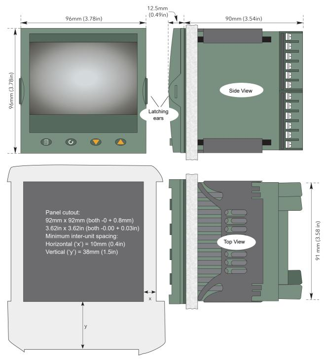
Figure 2 Mechanical installation details (standard case)
