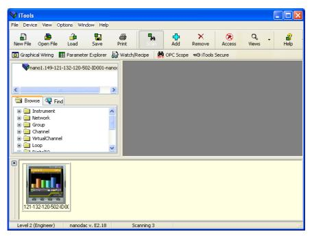
Figure 170 iTools initial window with one instrument detected
