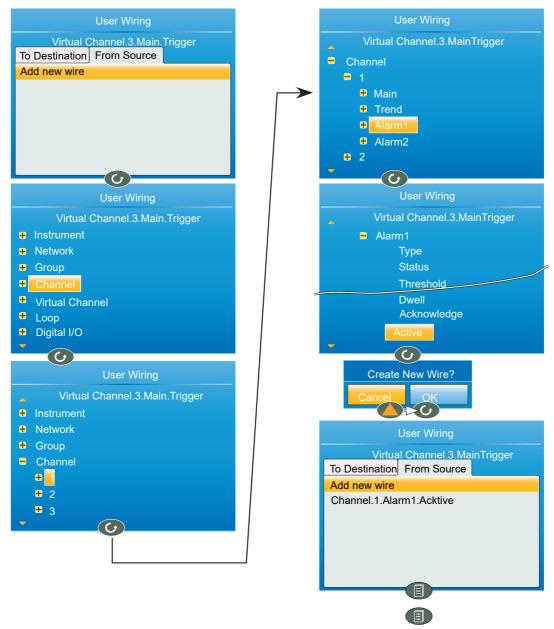
Figure 195 Wiring a counter: part 2
