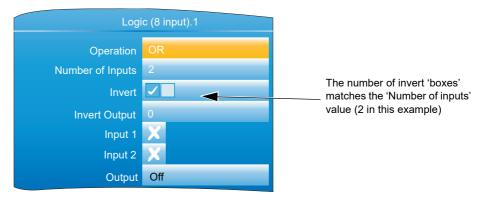
Figure 146 Eight input logic block configuration
