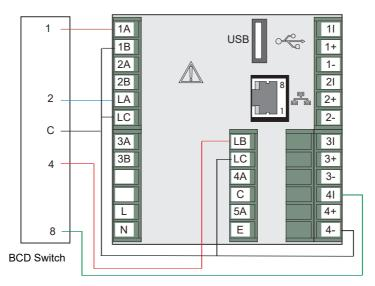
Figure 40 BCD Switch Physical Wiring
