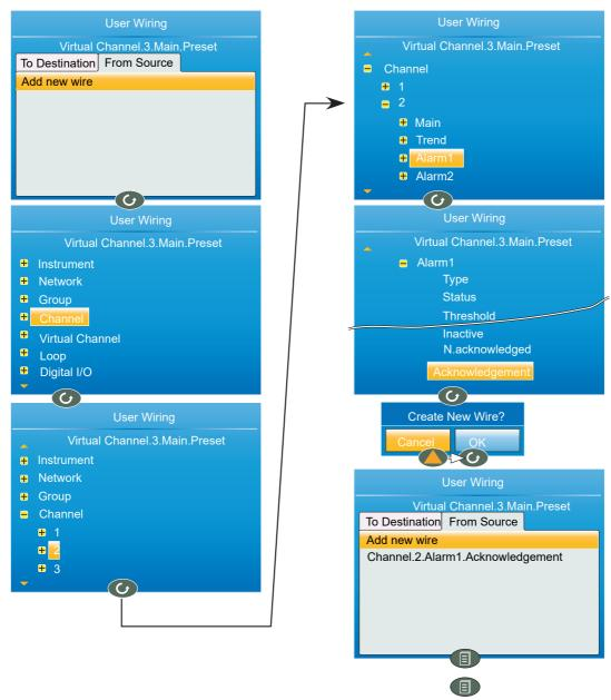
Figure 196 Wiring a counter: part 3
