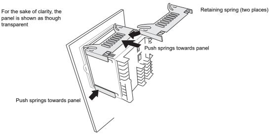
Figure 1 Securing the Instrument
