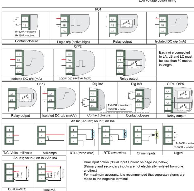
Figure 4 Connector locations and pinouts (rear panel)
