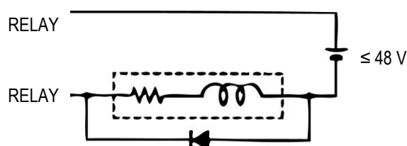
Figure 24: Spike Voltage Limitation for the Alarm Relay
