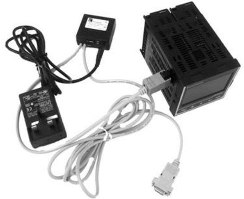
The 5-pin clip can be connected to the instrument either in or out of its sleeve. It is not necessary to power the instrument since power is supplied through the adaptor.
