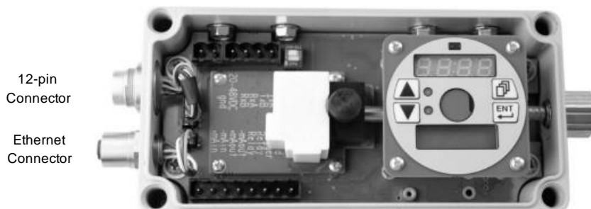
Figure 5-4: Electronics Housing with Outside 12-pin Connector
