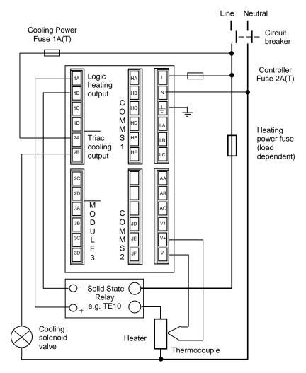
Figure 15: Typical wiring diagram, model 2408 controller
