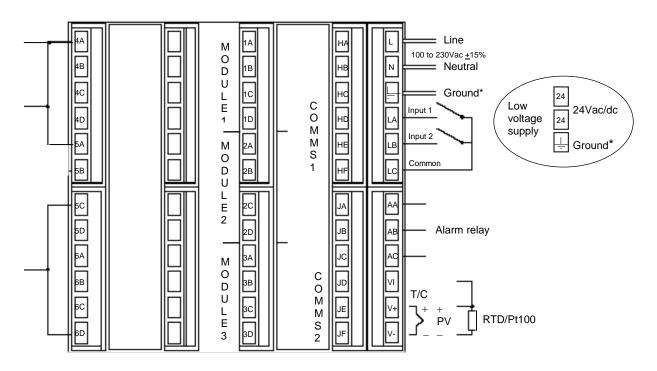
Figure 6: Rear terminal layout - Model 2404
