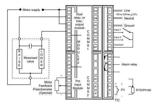
Figure 16: Motorised valve connections
