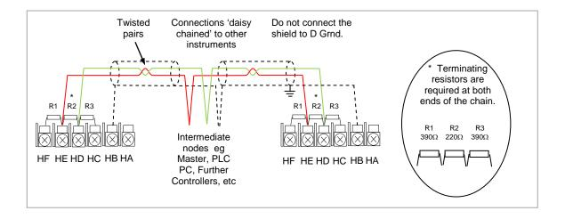
Figure 14: Profibus wiring example
