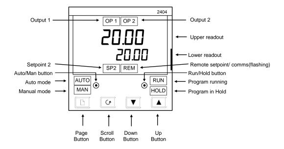
Figure 18: Model 2404 front panel layout
