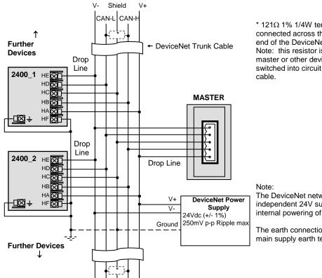
$^{\star}$  121 $\Omega$  1% 1/4W terminating resistor must be connected across the blue and white wires at each end of the DeviceNet trunk cable.
