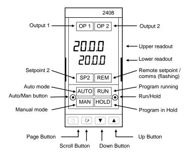
Figure 17: Model 2408 front panel layout
