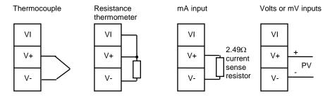
Figure 7: Sensor input connections
