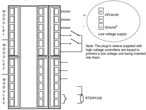
Figure 5: Rear terminal layout - Model 2408
