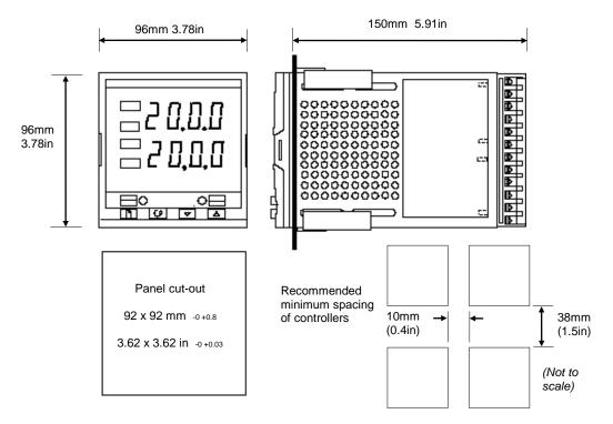
Figure 4: Outline dimensions of model 2404 controller
