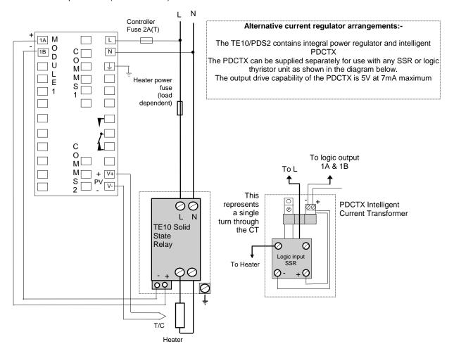
Figure 37: Connections for Mode 1 & 2
