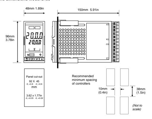
Figure 3: Outline dimensions of model 2408 controller
