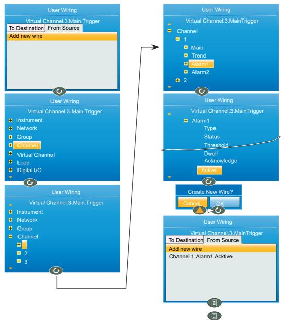
Figure 195 Wiring a counter: part 2
