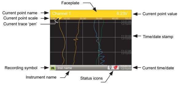
Figure 18 Vertical trend mode display elements
