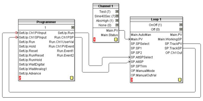
Figure 120 Programmer to Loop basic wiring
