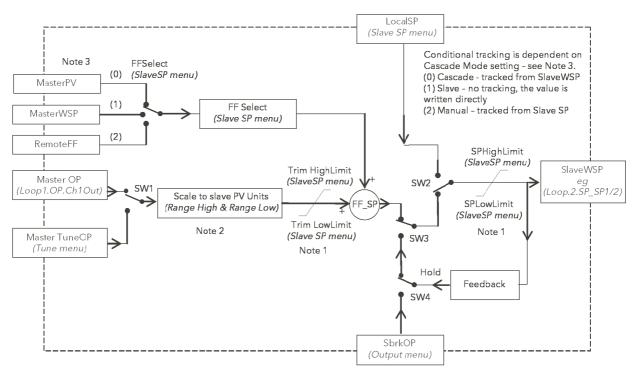
Figure 112 Cascade Trim Mode Block Diagram
