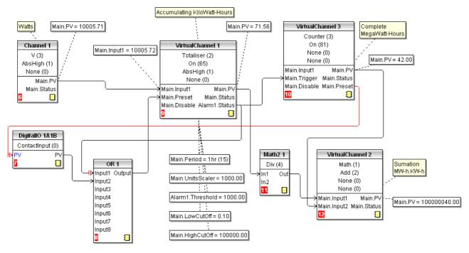
Figure 100 Linking a counter and totaliser
