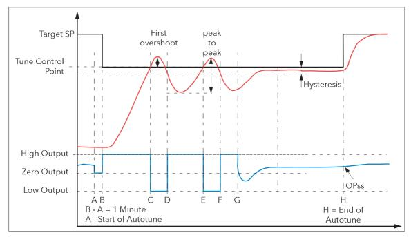
Figure 209 Autotune from below setpoint
