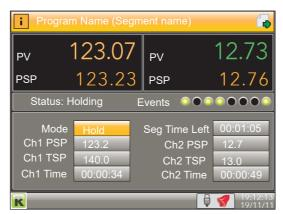
Figure 29 Two channel program in Hold mode
