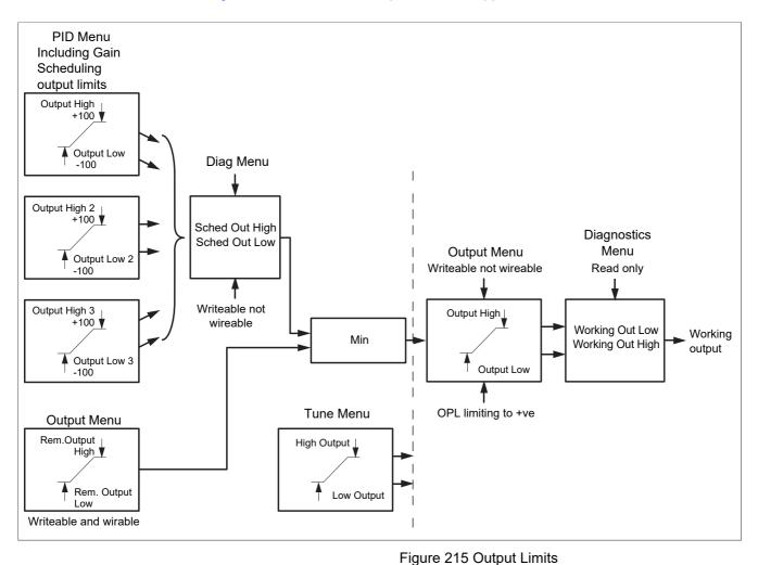
Figure 215 shows where output limits are applied.
