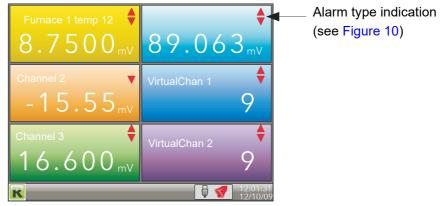
Figure 22 Numeric display mode (six enabled channels)
