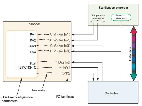
Figure 43 Typical steriliser application
