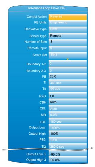
Figure 108 Advanced Loop Slave PID Menu (Typical)
