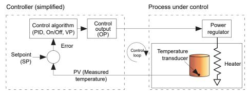
Figure 198 Control loop example
