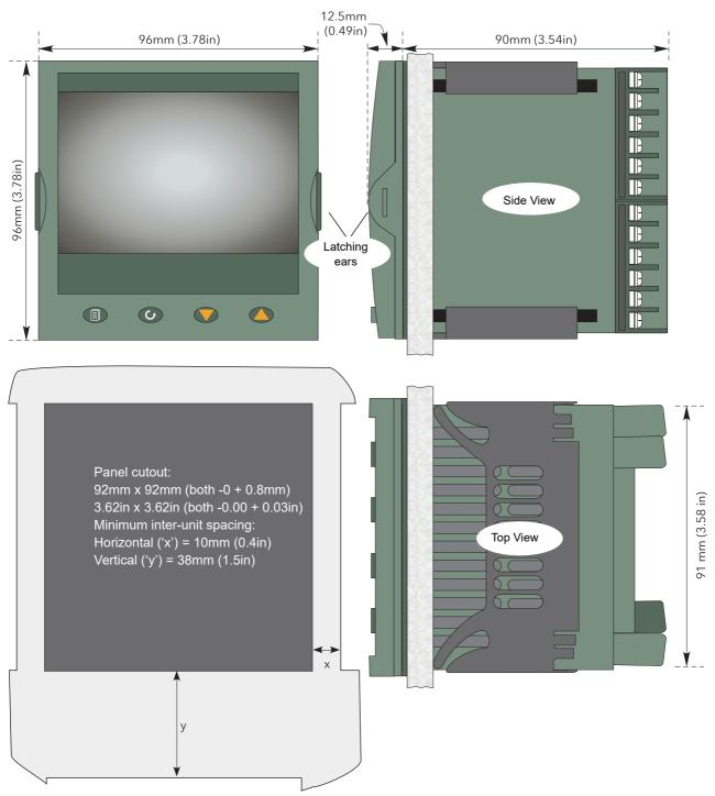
Figure 2 Mechanical installation details (standard case)
