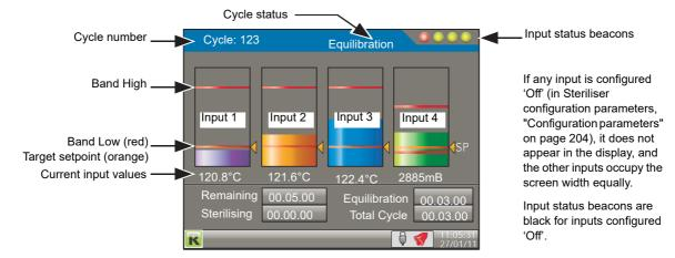
Figure 41 Steriliser display mode (typical) (four inputs)
