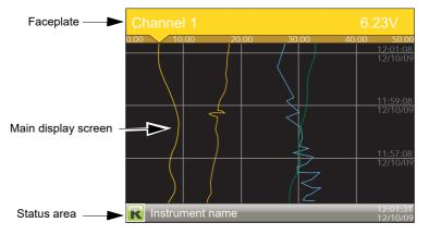
Figure 6 Display mode screen (vertical trend)
