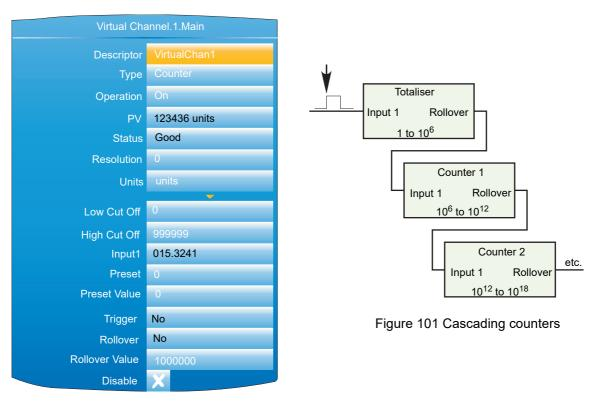
Figure 102 Typical Counter configuration
