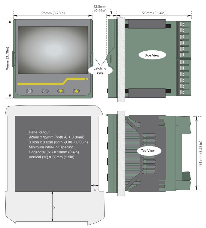
Figure 3 Mechanical installation details (wash down case option)
