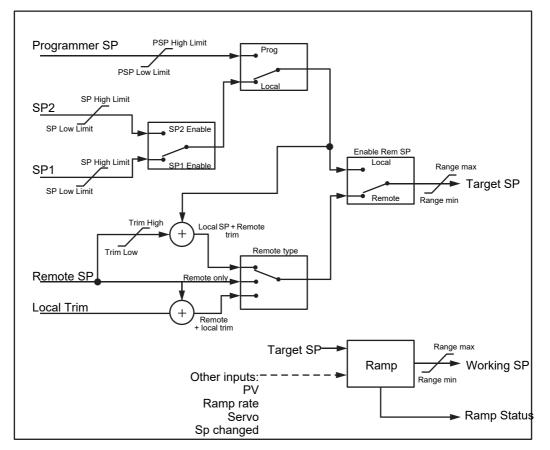
Figure 213 shows the function block schematic.
