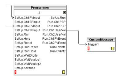
Figure 35 iTools example showing Ch1 UserVal being used to trigger custom message 1.
