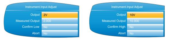
Figure 78 Low and High adjust point displays
