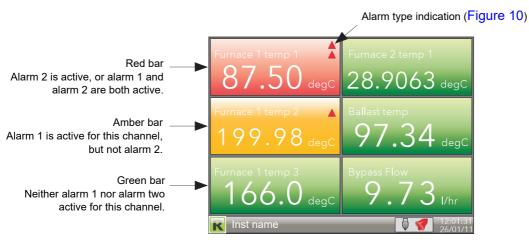
Figure 24 Alarm panel display (six channels)
