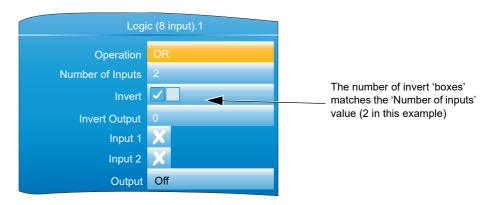
Figure 146 Eight input logic block configuration
