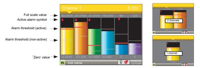
Figure 20 Vertical bargraph display mode
