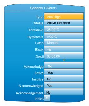
Figure 93 Typical alarm 1 configuration menu
