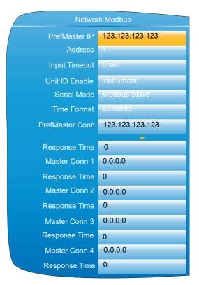
Figure 84 Modbus TCP configuration menu
