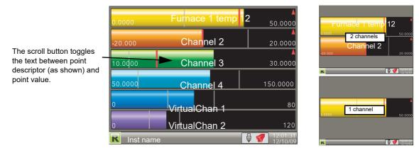
Figure 21 Horizontal bargraph mode
