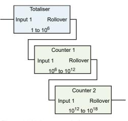
Figure 98 Using cascaded counters to expand the totalisation range.
