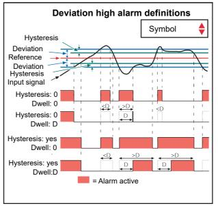
Figure 95 Deviation alarm parameters
