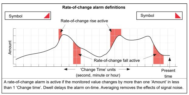
Figure 96 Rate-of-change alarm parameters
