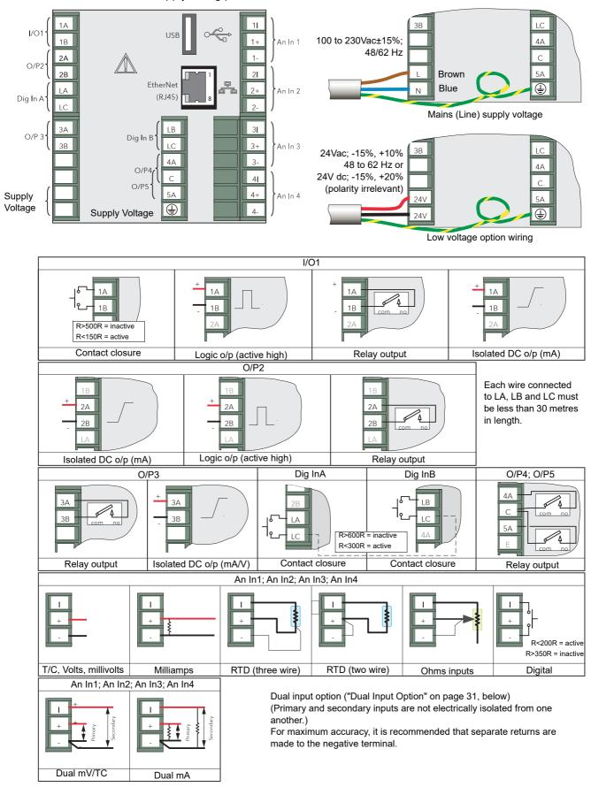
Figure 4 Connector locations and pinouts (rear panel)
