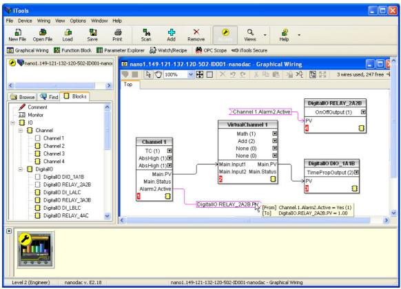
Figure 171 Graphical wiring Editor
