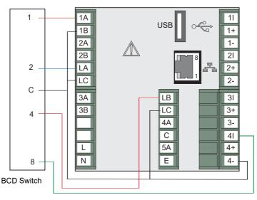
Figure 40 BCD Switch Physical Wiring
