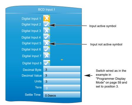
Figure 144 BCD block configuration
