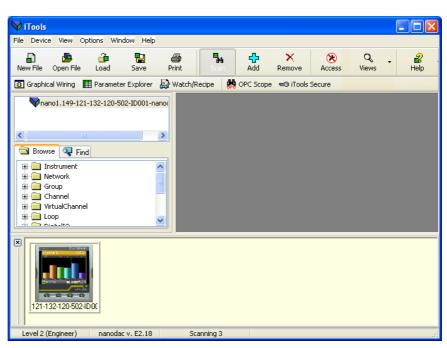
Figure 170 iTools initial window with one instrument detected
