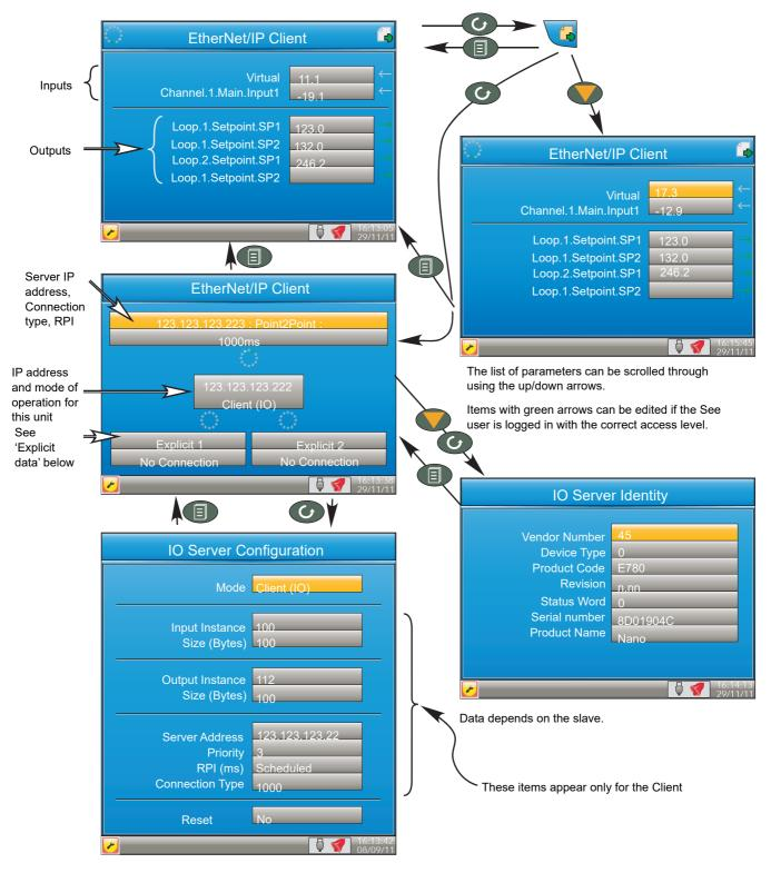
Figure 49 Typical EtherNet/IP display
