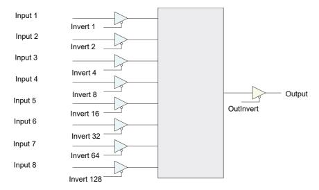
Figure 147 Logic (8 input) block schematic
