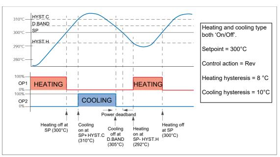
Figure 218 Deadband ON set at 50% of Cooling.
