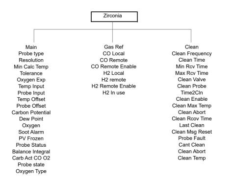
Figure 134 Zirconia probe configuration layout.
