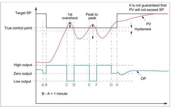
Figure 205 Autotune heat/cool process
