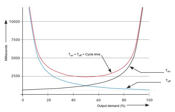
Figure 220 Time proportioning curves (Minimum on time = 625ms) **Note:** For this instrument, only 'Min on time' is configurable
