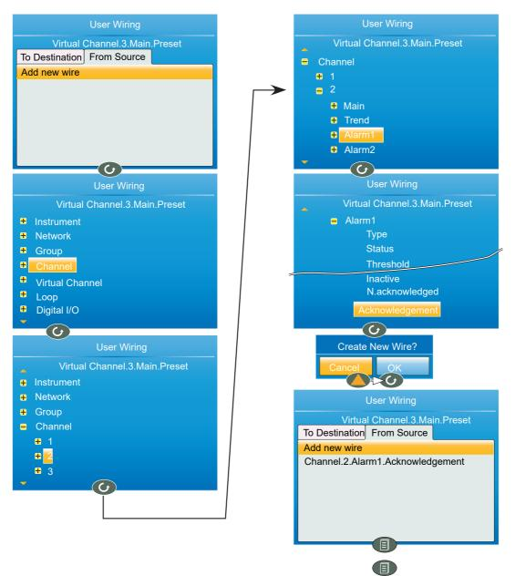
Figure 196 Wiring a counter: part 3
