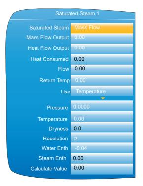
Figure 139 Saturated Steam configuration
