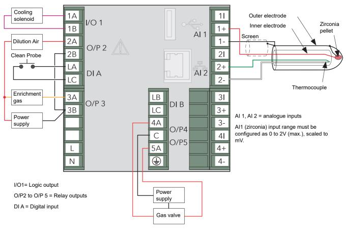
Figure 136 shows a typical wiring arrangement for a Zirconia probe.
