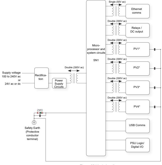
Figure 224 Isolation diagram
