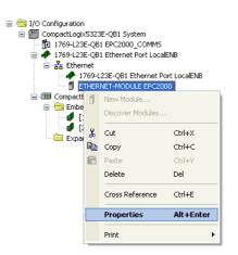
5. Set Requested Packet Interval (RPI) using Module Properties 'Connection' tab making sure that it is within 50 to 3200ms then click OK.
