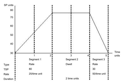
The example above shows a simple three segment program in which the Target Setpoint (TSP) increases at a controlled rate of 25/time unit to a value of 75. It then dwells at that setpoint for two time units before decreasing to 30 at a controlled rate of 50/time unit.
