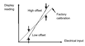
The procedure is exactly the same as shown in the previous section. For the minimum input set the 'CalValue' to the reading required on the controller as shown in the Low offset in the diagram above.
