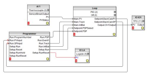
The figure below shows a simple soft wiring diagram for a programmer.
