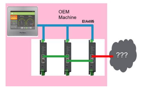
It should be noted that EIA485 communications is given priority over Ethernet communications, however, EIA485 is slow in comparison and therefore consideration should be given to the latency between the EPC2000 Programmable Controller and the HMI via EIA485.
