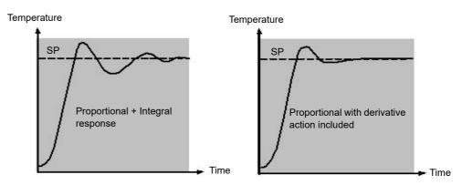
The derivative modifies the output to reduce the rate of change of the difference. It reacts to changes in the PV by changing the output to remove the transient. Increasing the derivative time will reduce the settling time of the loop after a transient change.
