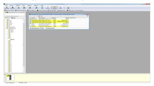
3. To send the write request, set the 'Send' parameter. The Status will go to 'Pending(13)' briefly before going to 'Success' when the parameter has been written. If the write has failed then the Status will show the reason for the failure.
