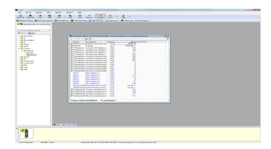
4. From iTools, place the instrument out of Config to restart the instrument and initialize new comms settings.
