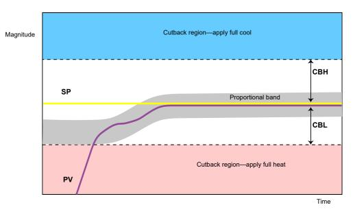
**Note:** Because cutback is a type of non-linear controller, a set of CBH and CBL values that are tuned for one particular operating point may not be satisfactory for another operating point. It is advisable therefore not to try to tune the cutback values tightly, or otherwise to use gain scheduling to schedule different values of CBH and CBL at different operating points. All the PID tuning parameters can be gain scheduled.
