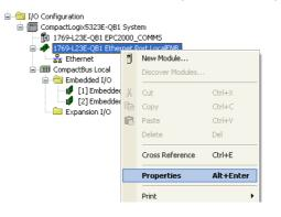
5. In the Module Properties window, configure the IP address and click OK.
