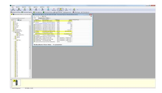
5. Configure a second slave by setting the device's IP Address and unit ID.
