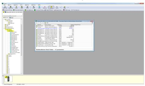
1. From iTools, place the instrument in Config mode and open: ModbusMaster>Slave1>Main to configure the first slave. 2. Configure the slave's IP Address and unit ID.
