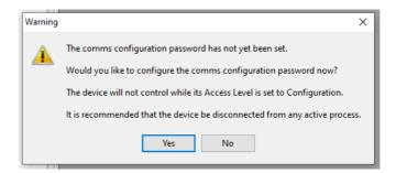
Informing the user that they need to configure the Comms Configuration password before being able to proceed. Selecting 'Yes' will automatically launch the iDevPWSetup tool.
