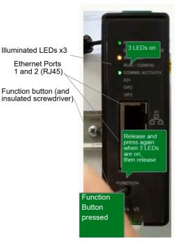
**Note:** Make sure that the controller and PC which is running iTools are on the same subnet.
